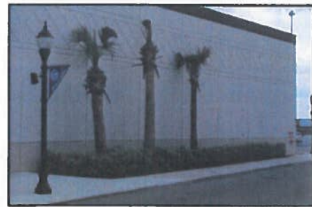
Don't do this: Blank, monolithic walls and a flat roof along a pedestrian frontage that does not have windows, doors, or other pedestrian-scale treatments.
